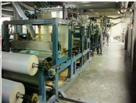
In House GRP Sheetting
